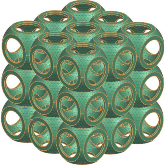
Figure 3.4.3 Fem file of a compression specimen model. The 3D mesh of the part is represented in green
