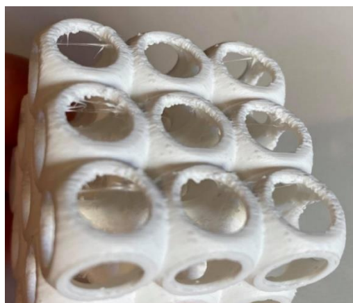
Figure 2.8.12 Visible strings inside the part
