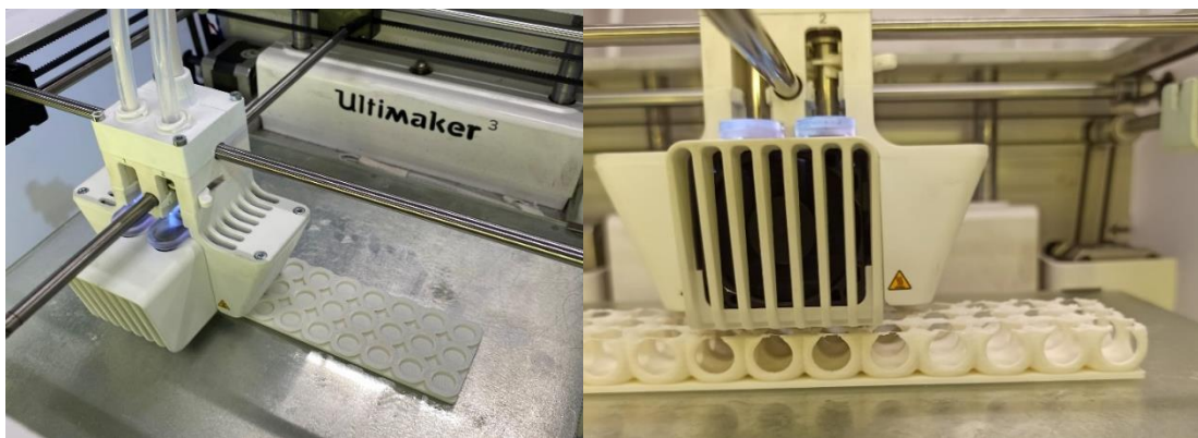
Figure 3.2.7 Examples of bending specimens being printed
