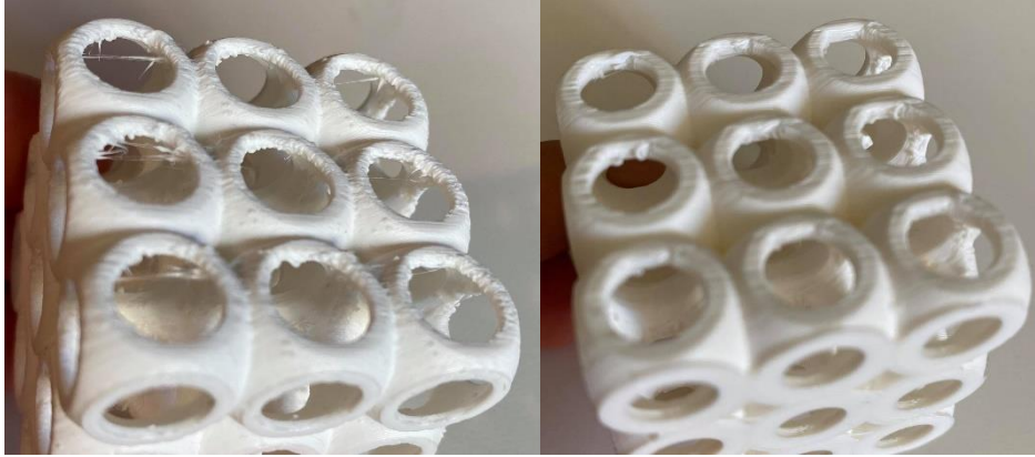
Figure 3.2.5 Evolution of stringing in the specimens, after the activation of “z-hop” and “avoid printed parts” parameters. On the left, a part with some strings, and on the right, a part with almost zero strings
