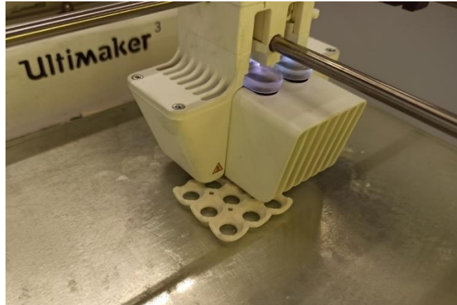
Figure 3.2.6 Example of a compression specimen being printed
