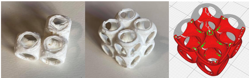
Figure 3.2.2 Specimens tested to define the final dimensions (scale factor)
