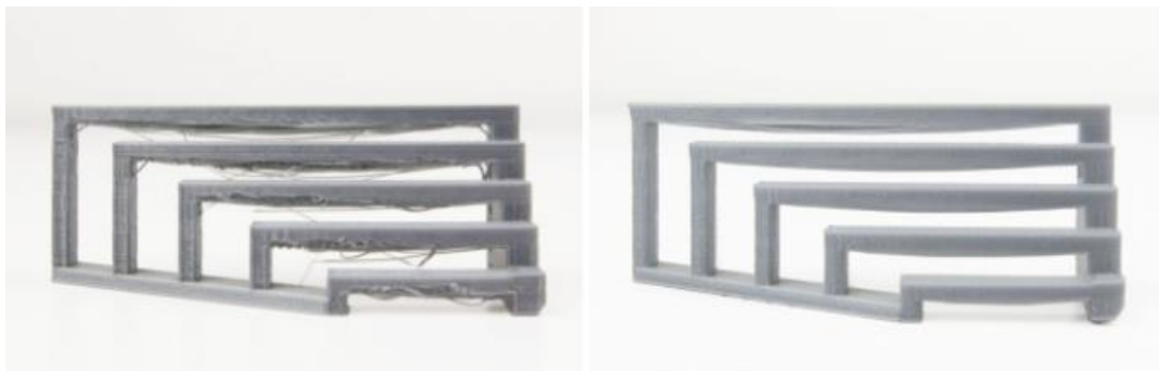
Figure 2.8.7 Example of a part with, on the left side, and without bridging, on the right side [34]
