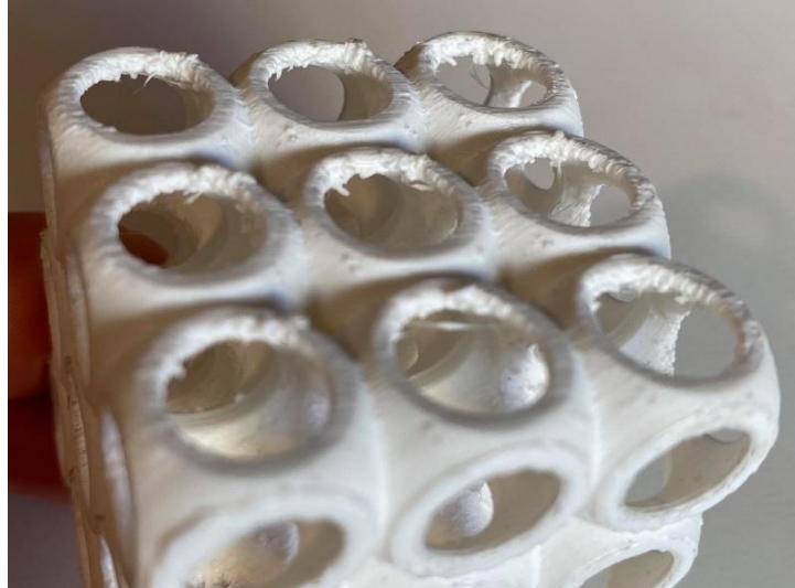
Figure 2.8.8 Example of a part with curly filaments in the top of the holes due to overhangs
